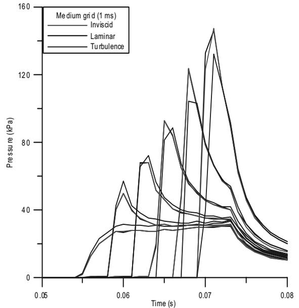
Fig. 3 Comparison of pressures (viscosity effect)
