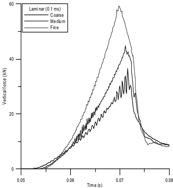
Fig. 5 Comparison of vertical forces (grid size effect)
