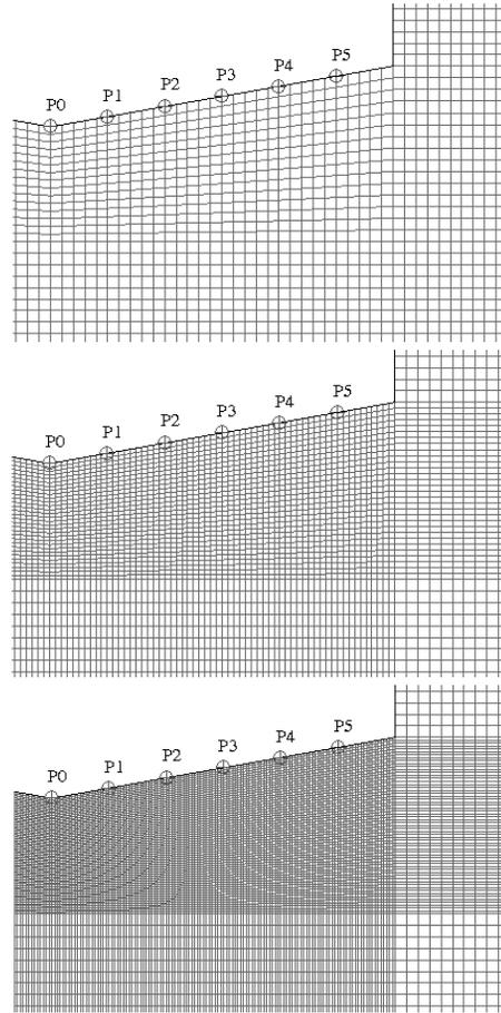
Fig. 2 Three different grid system: coarse (top), medium (middle) and fine (bottom) grid
