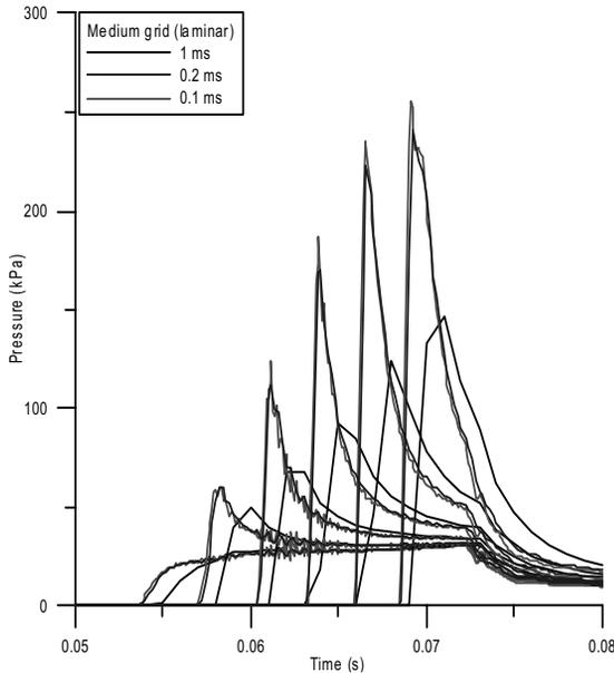
Fig. 8 Comparison of pressures (time step size effect)
