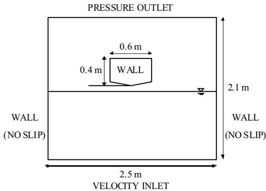
Fig. 1 Schematic view of the wedge model, the calculation domain and the boundary conditions
