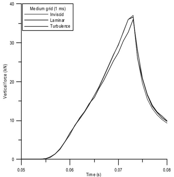
Fig. 4 Comparison of vertical forces (viscosity effect)
