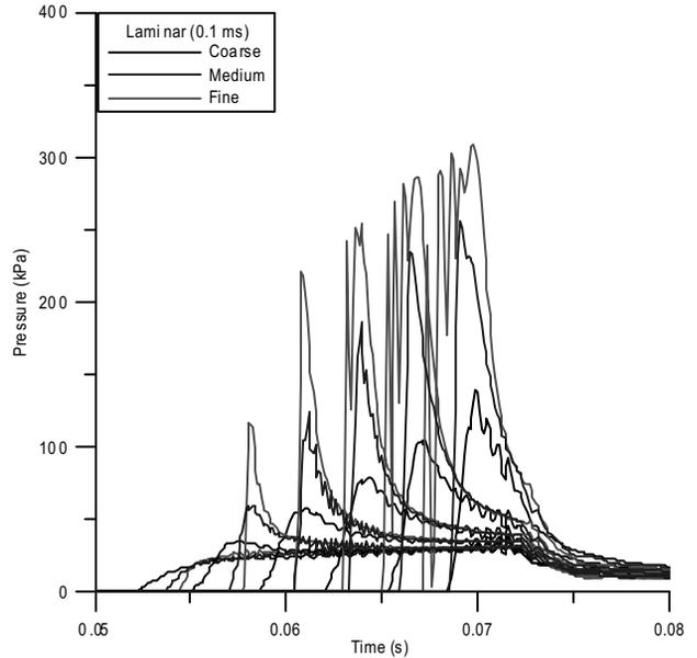
Fig. 6 Comparison of pressures (grid size effect)
