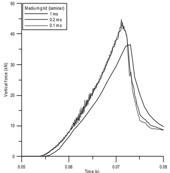
Fig. 7 Comparison of vertical forces (time step size effect)
