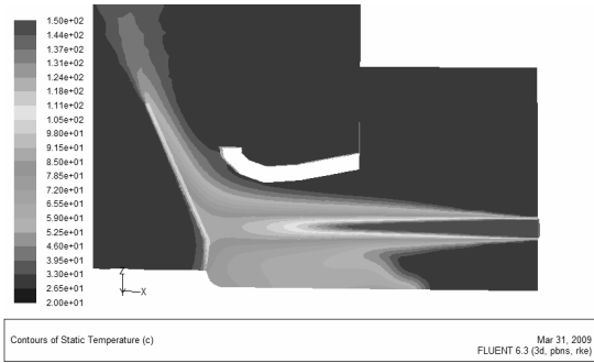
Fig. 12 Closed ventilation type II (temperature)
