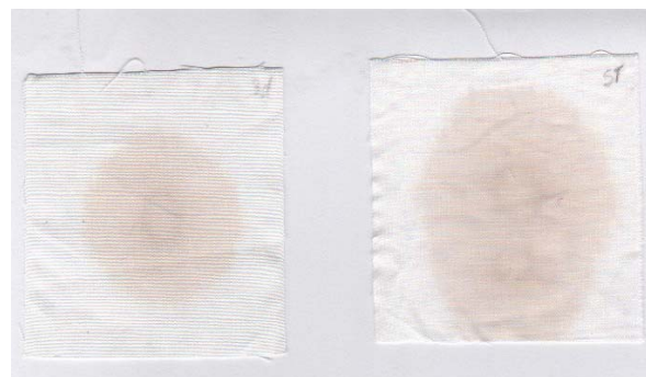
Figure 5. Staining of engine oil on chitosan treated fabric (left) and on untreated fabric (right) [5].
