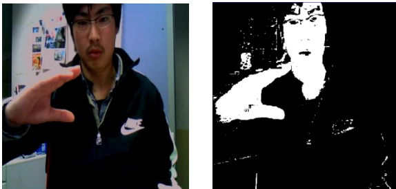
Fig 3: Left: Camera frame and composed CG. Right: Skin color detection from camera frame
