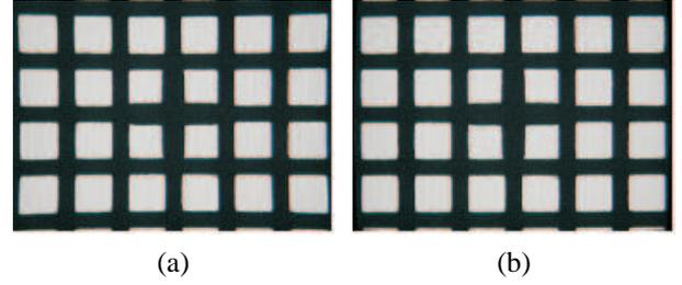
**Fig. 2.** Compensation of the grid image . (a) Deformed image (sigmoid distortion obtained by an optic-microscope with  $\times 100$ ). (b) Corrected image ( $k_1 \approx -2.1 \times 10^{-6}$  and  $k_2 \approx -9.9 \times 10^{-9}$ ).
