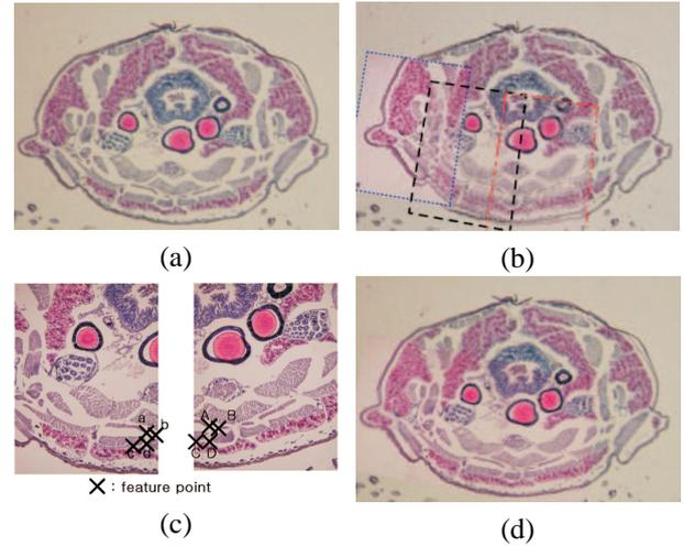
**Fig. 4.** Correction and registration of the trichoptera image. (a) Corrected low-magnification image ( $\times 100$ ). (b) Registration of high-magnification images ((b)-(d) of Fig. 3) without correction (MSE = 26.6dB). (c) Example of feature points a and b ((c) and (d) of Fig. 3). (d) Registration of corrected images (coefficients from the feature points in (c) (MSE = 24.6dB).
