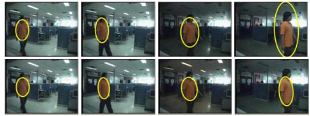
Figure 8 Tracking result using only color cue (top) versus using both color and shape cues (bottom) on an indoor sequence with changing illumination.
