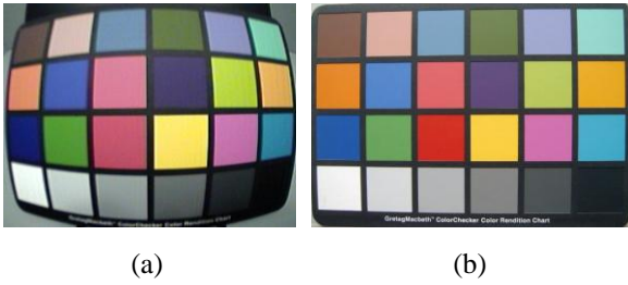
Fig. 3: Examples of camera images: (a) image obtained from vehicular rear-view camera and (b) image obtained from regular digital camera.
