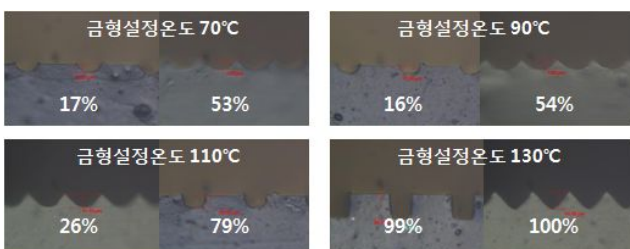
Fig. 5 Replication results for different mold temperatures (End region of the cavity)
