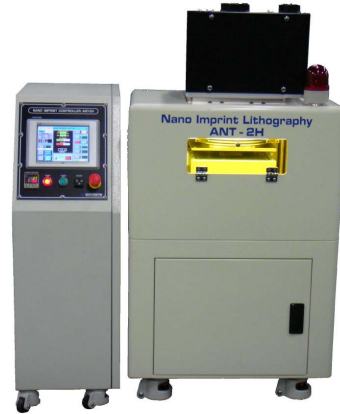
Fig. 1 Developed hybrid nanoimprint equipment by KIMM for 2 inch wafer area (ANT-2H).
