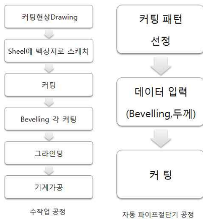
Fig. 1 Compared Flowchart with Manual Process and Automatic Pipe Profiling cutting M/C
