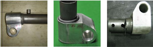
(a) bending failure (b) buckling failure (c) torsional failure
