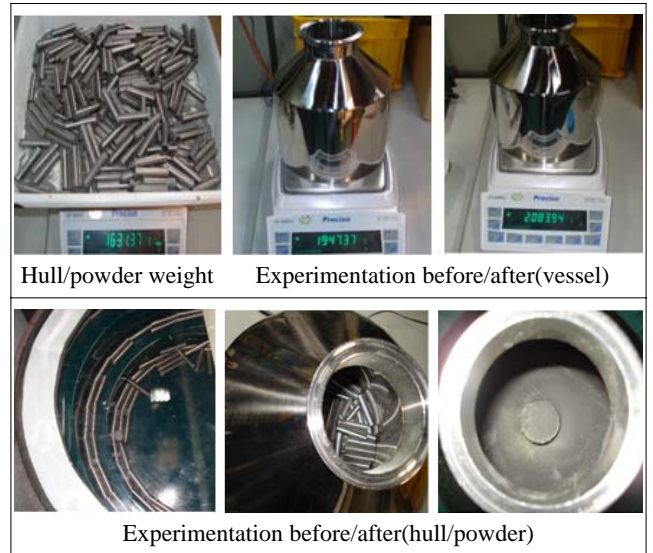
Fig 6. Test results of auto-separation device for hull and Powders.
