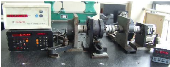
Figure.5 Transmission Angular Error Test Rig
