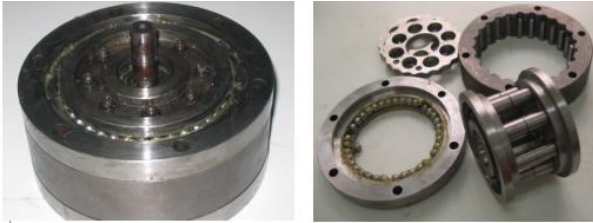
Figure.4 Double disc conic cycloid reducer
