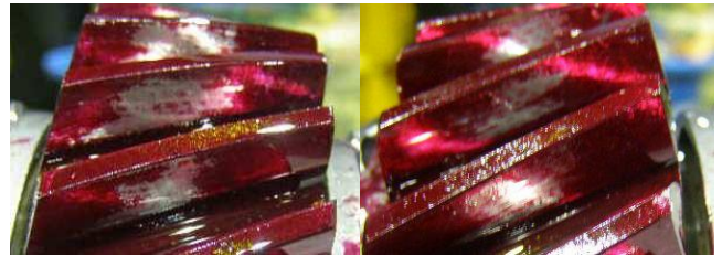
(a) Drive gear – left and right flank
