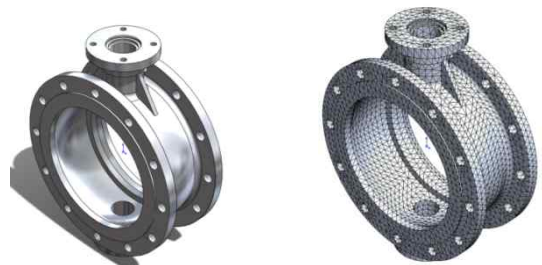
Fig. 1 Model of butterfly valve body for Structure analysis(SUS304)
