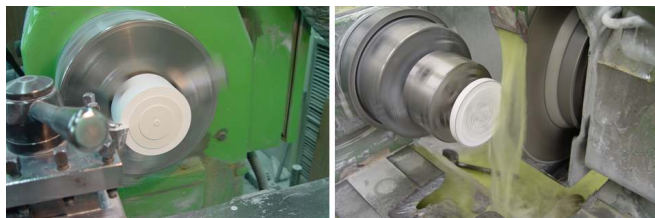
Fig.5 Mechanical machining process of ceramic isolation plate
