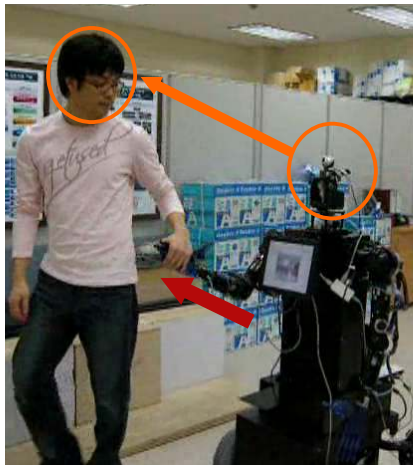
Fig. 3 Interaction for Following Human using Haptic and Face Detection Methods
