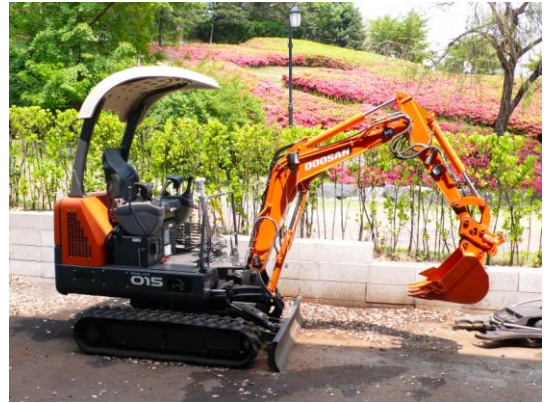
Fig. 2 Hydraulic excavator (SOLAR015) equipped with PVC and inclinometer sensors
