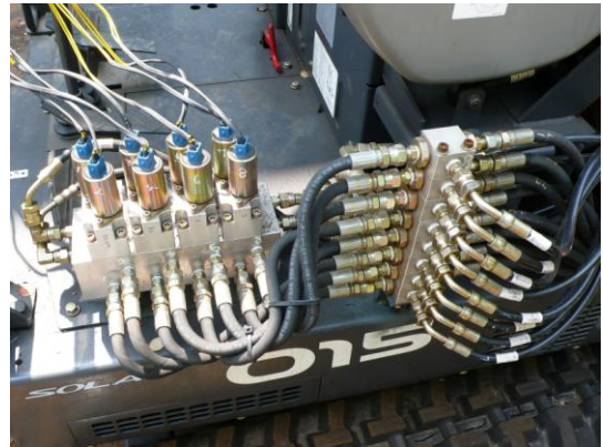
Fig. 3 Proportional valve control system
