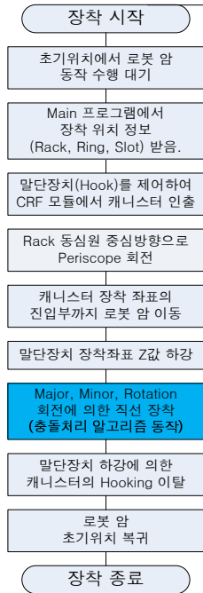
Fig. 3 Flow chart of robot arm control program
