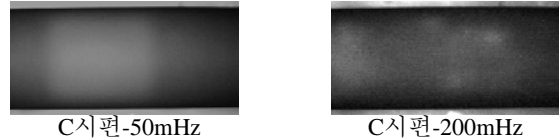
Fig. 6 Defect detection of Pipes by Frequency
