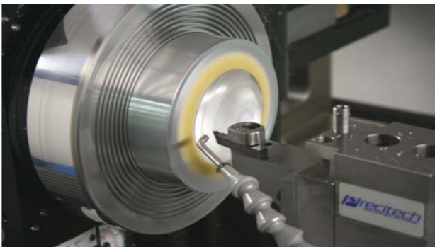
Fig. 4 Ultra precision machining of G5 lens
