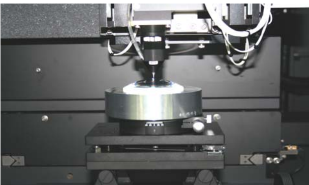
Fig. 5 Measurement of G5 Aspheric surface (UA3P)
