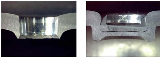
Fig. 3 Clinching geometry of neck fracture mode
