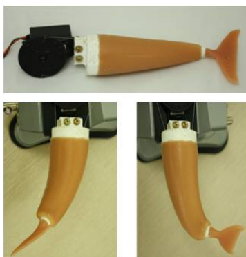
Fig. 5 The completed actuation part of the robotic fish (top), Motion of the robotic fish (bottom)
