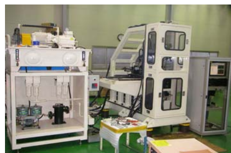
Fig. 5 Developed valve balance tester
