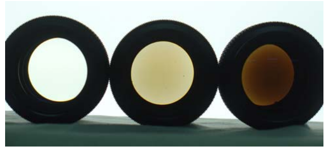
Fig. 2. Lens degradation by color center after high dose rate gamma irradiation. (left: before, center: after 4kGy, right: after 8kGy)
