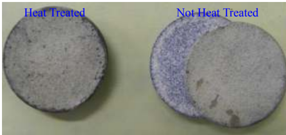
After thermal shock test(1,100℃/30min, 21cycle)
