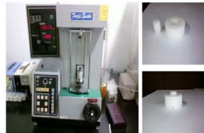
Fig. 2 Experiment device for spring compression
