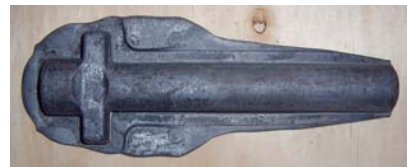
Fig. 7 Plunger product from finisher process
