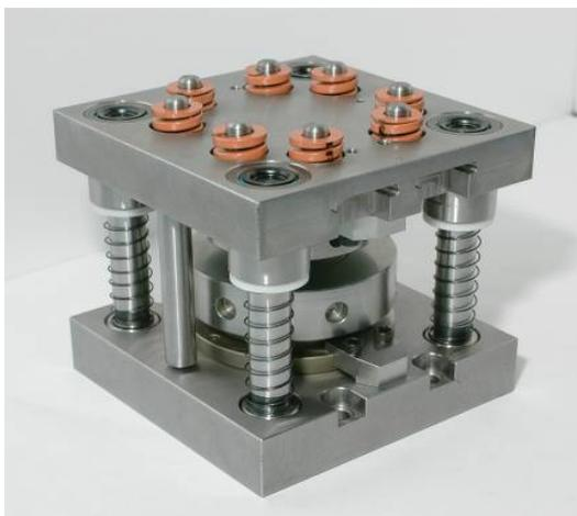
Fig 5. Die set and spring structure
