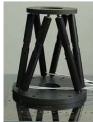
Fig. 1. Photograph of the developed Stewart platform.
