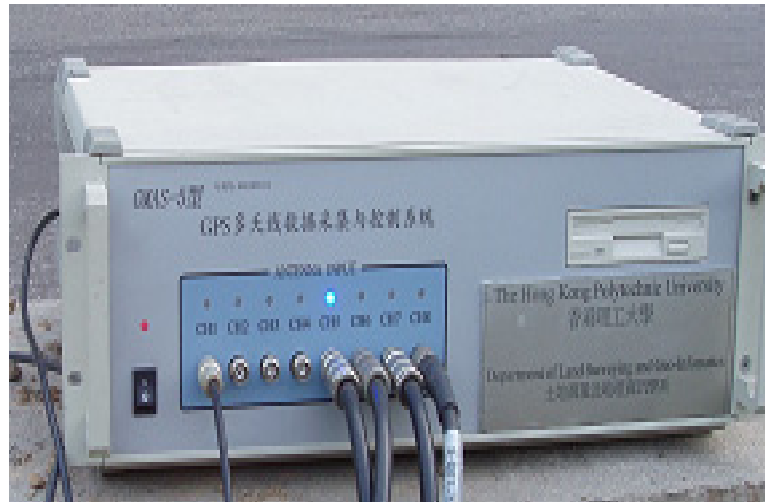
Figure 2. GPS multi-antenna control unit
