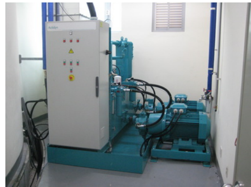
Figure 9. Hydraulic power supply for the shaking table
