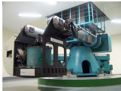
Figure 6. Beam centrifuge at KAIST
