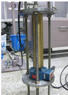
Fig. 10 Loading transfer verification test
