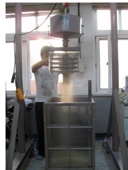
Fig. 19 Spreading sand for making dense ground
