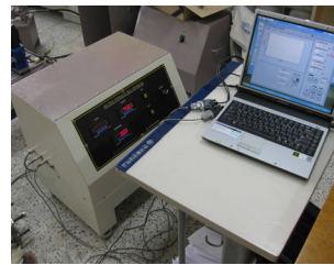
Fig. 9 Loading control and data collection apparatus
