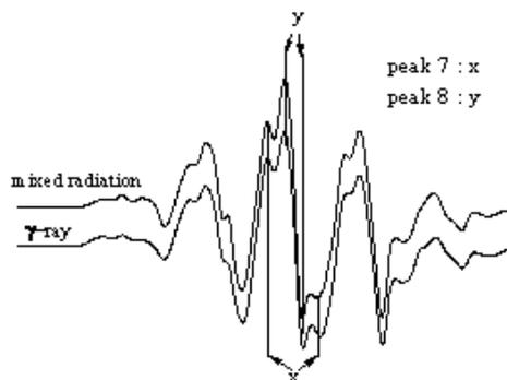
Fig. 1. Signal of alanine pallet irradiated with gamma-ray(1,500Gy) and mixed radiation measured with reference of Co-60(1,800Gy), showed ratio difference.
