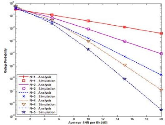
Fig. 1 Outage Probability of repetition coding for  $R = 0.5$  with different values of  $N$ .
