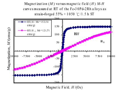
Fig. 2. Magnetization ( $M$ ) versus magnetic field ( $H$ )  $M$ - $H$  curves measured at RT of the Fe-30Pd-2Rh alloys strain-forged a 55% reduction in thickness and annealing at 1050 °C for 1.5 h then quenching in ice brine.  $H \perp$  denotes the magnetic field was applied perpendicular to the sample's cross section.
