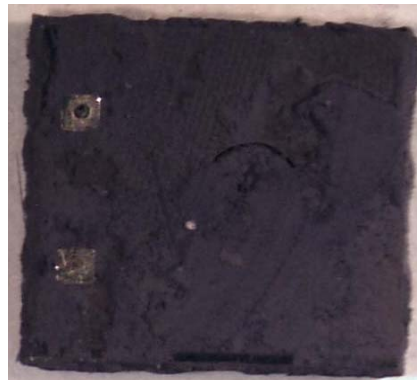
Fig. 2. Fabricated power inductor.
