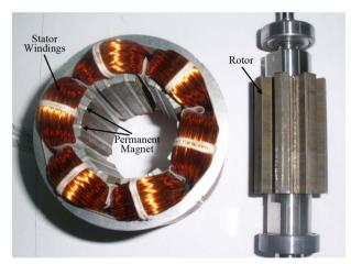
Fig. 1. The constructed inset type FRM.
