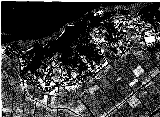
Figure 3. Geo-rectified IKONOS image overlaid with national digital map. The IKONOS image was geo-rectified using the GCPs extracted from the TerraSAR-X data.
