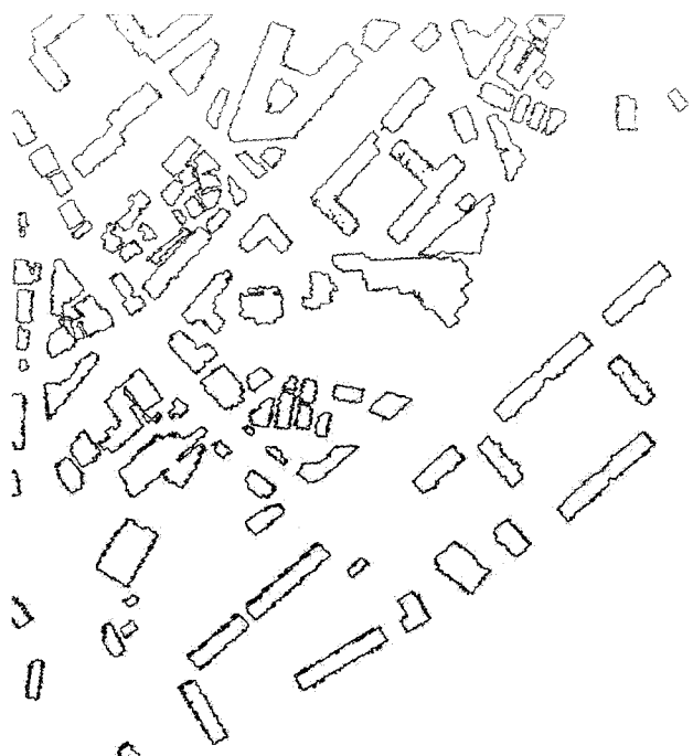
Figure 9. The extracted building from P-NDSM
