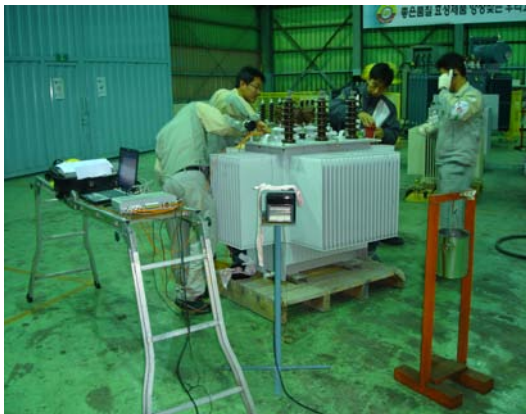
Fig.3 Experiment of temperature rise of the transformer
