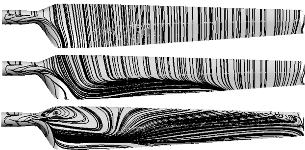
Fig. 6 Suction side surface streamlines, 7m/s, 10.02 m/s, and 20.13m/s(from top to bottom, k-ε model)
