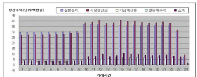
Fig. 12 Profit increase when constrained power generation was decreased timely as heat supply decreased
