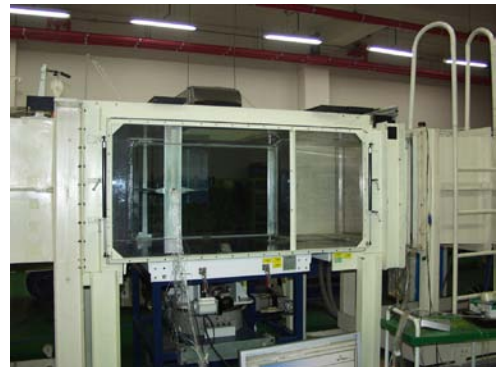
Fig. 6 1m x 1m Subsonic Wind Tunnel Test
