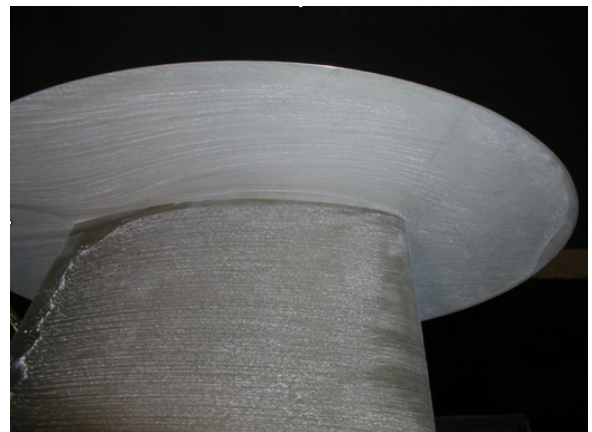
Fig. 12 Flow Visualization ( M=0.6 )
