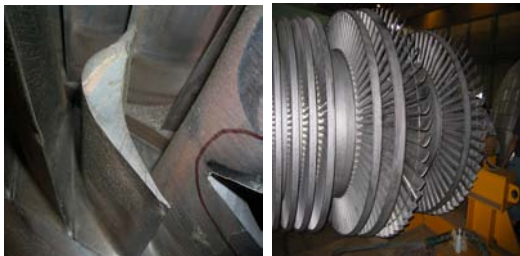
(Fig. 5 Photograph before and after replacing high pressure turbine blade)
