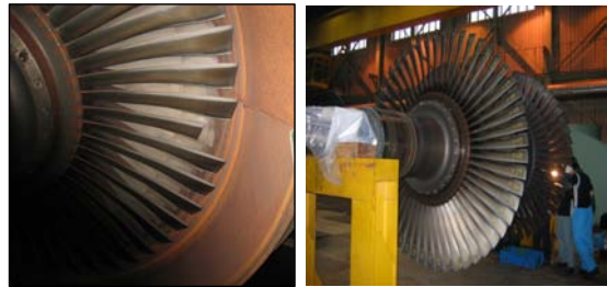
(Fig. 6 Photograph before and after replacing low pressure turbine blade)
