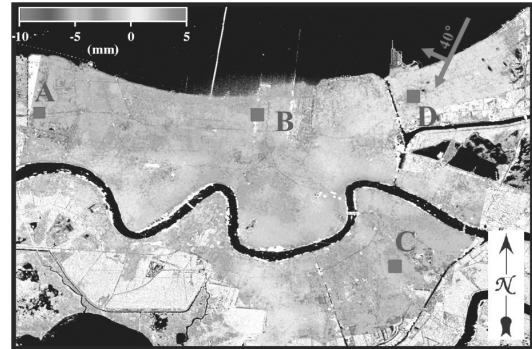
Fig 3. LOS velocity map at New Orleans during 2005-2007. Arrow indicates flight and LOS direction. Look angle is about 40^\circ .
