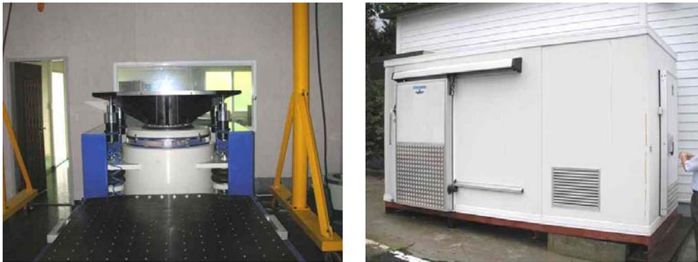
Figure 2. Vibration Tester and Environmental Chamber.
