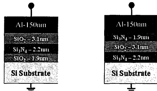
(a) ONO stacked structure (b) NON stacked structure
