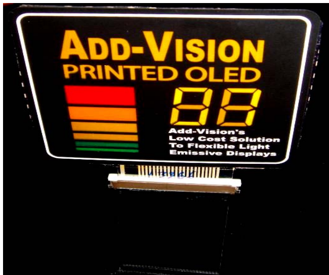
Figure 4 Example of an Add-Vision OLED Display as shown at SID, laminated in between two Barix Barrier Films.
