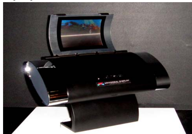
Fig 3. Flexible AM Matrix Display by LG.Philips and UDC on metal foil substrate, encapsulated with Vitex Barix encapsulation as shown at SID.
