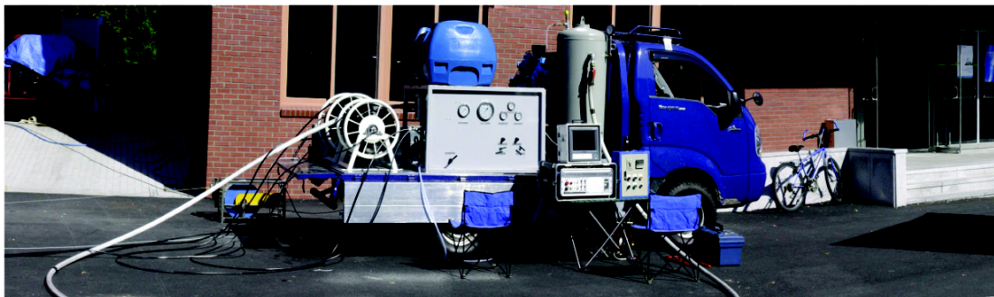
Fig. 4 Photograph of the recent hydrofracturing system, which can be operated by self-electric power and self-compressed air power (Developed by KIGAM & Dyke, Co., Patent no.; 10-0646584).
